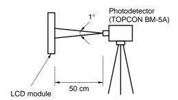
3. The contrast ratio is calculated by using the following formula.
