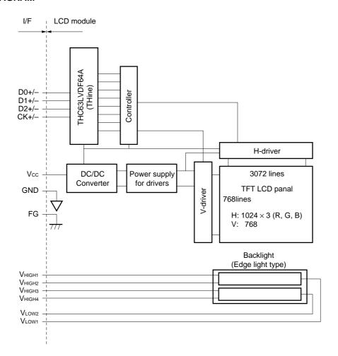
**Note** GND is connected to FG (frame ground) in the LCD module. These grounds should be connected in customer equipment.
