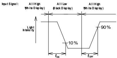
$t_{\rm ON}$ : Turn on time is the time for a photo detector output waveform to go from its maximum value to 10% of its maximum.
