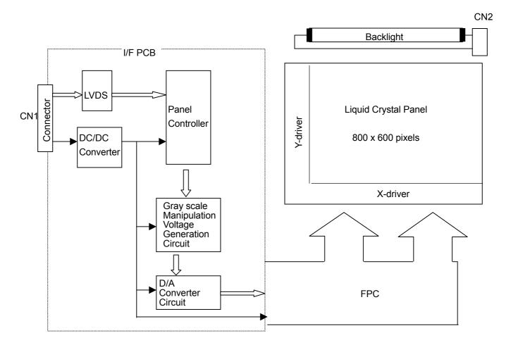
Note 1) Build up LCD drivers on the glass substrate
