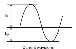
Unbalance rate =  $| I_p - I_{-p} | / I_L \times 100$  (%) Wave-height rate =  $I_p$  (or  $I_{-p}$ ) /  $I_L$
