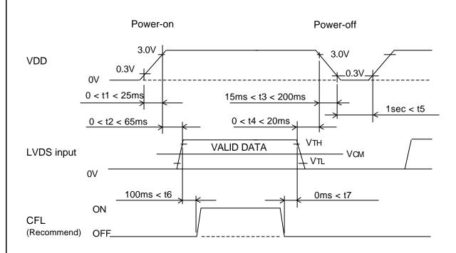
When the power is off, LVDS input must be kept at either low level or high impedance.
